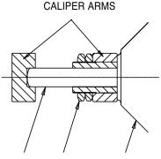
PUSHROD LOCKNUTS THRUSTER
