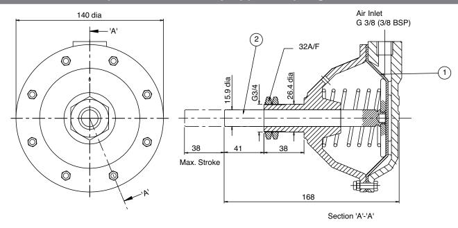
This range of pneumatically operated brakes uses dry and filtered compressed air at pressures up ot 7 bar. Pneumatic brakes require a control valve which may be operated either manually, or by pneumatic or electrical signal.
