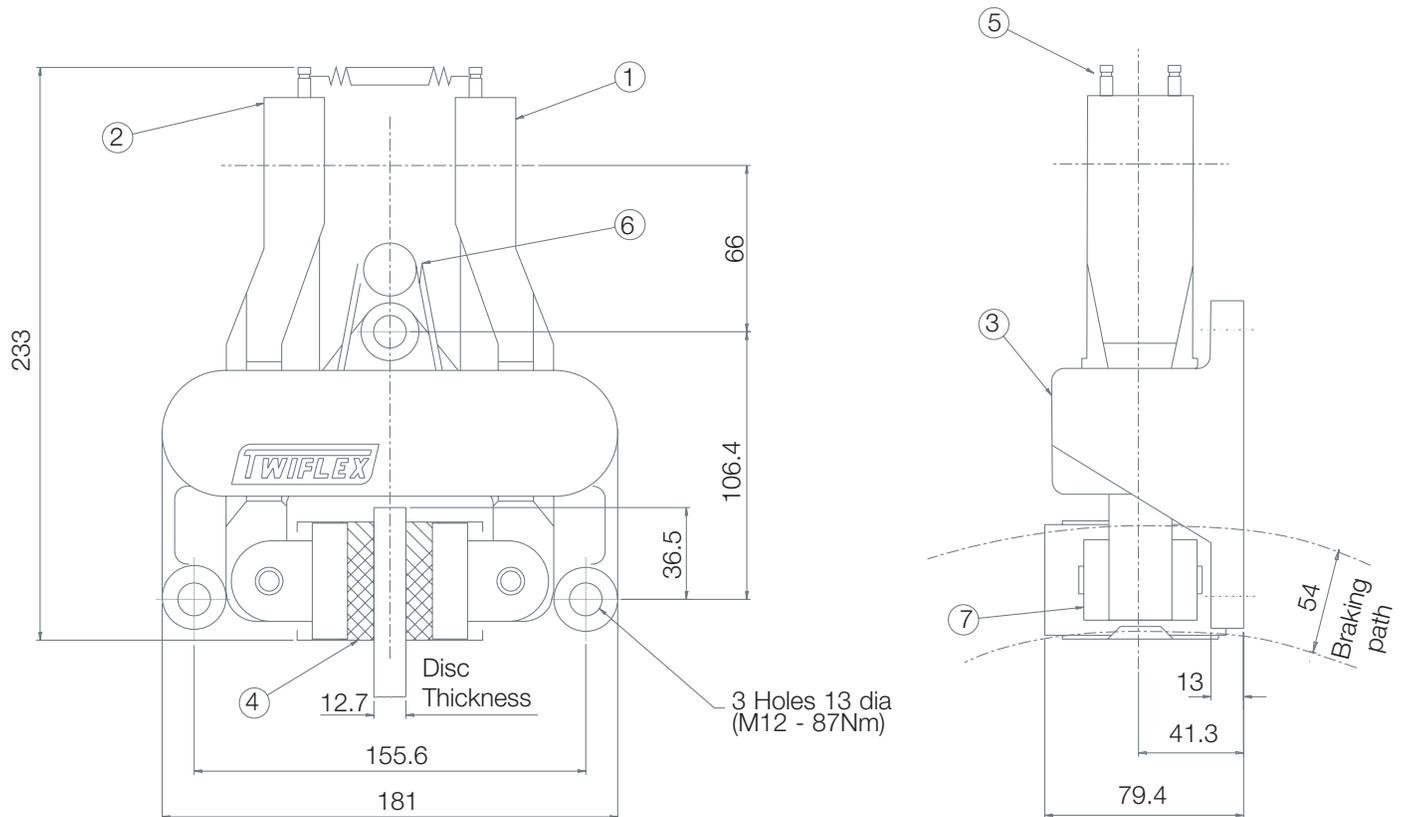
**Disc Brake Caliper Part Number 6780413**
