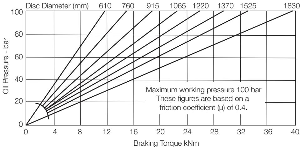
These are typical performance figures for fully bedded and conditioned brake pads. For bedding-in and conditioning see publication M1060. When used with standard Twiflex brake discs an appropriate service factor should be applied when designing the braking system, and in case of brakes used for holding duties or in wet conditions this should be not less than 2.0.
